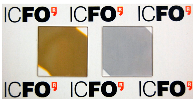
Figure 8. Pictures of 6 nm Ag film without (left) and with seed layer (right) 24 h and 4 months after deposition respectively. Freshly deposited Ag films without seed layer look exactly the same as the Ag film with seed layer 4 months after deposition as shown in the picture.
